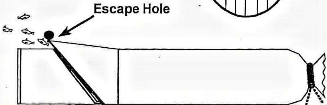
Hickman's Modified Sea Eagle II BRD. A. Schematic view showing attachment of device to trawl body, method of fish escapement, and door mechanism. B. Schematic showing location of the Modified Sea Eagle II BRD on the trawl.
